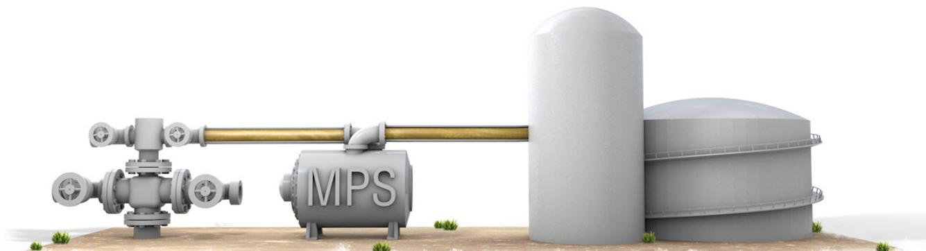
In field separation, the wellhead facility exerts a required pressure on the well to drive the production fluid through a local separation/ takeaway processing battery.
