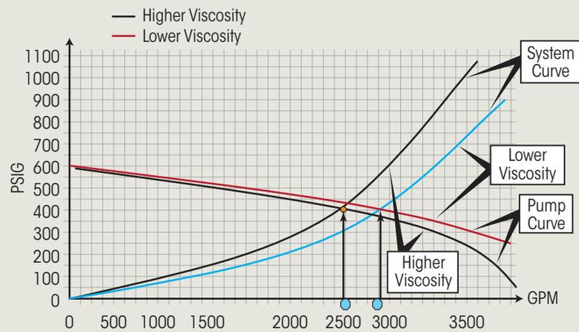
economical choice when liquid viscosity changes, but flow volume remains constant. The efficiency of centrifugal pumps drops rapidly when viscosity is outside the optimal range (also known as the Best Efficiency Point, or BEP), whereas positive displacement pumps are less susceptible to these fluctuations (Figure 2).
