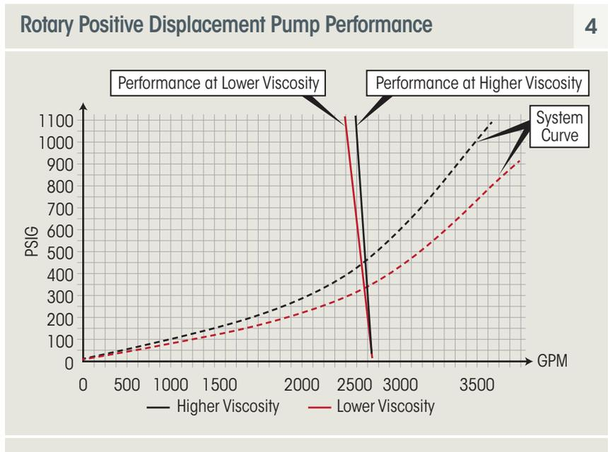
lift capability, which provides an operation margin for “upset” conditions, such as during startup when the liquid may be cold and more viscous or when there is an extended distance to the supply reservoir. This operation margin allows the use of smaller supply piping, reducing component costs and a simpler design.
